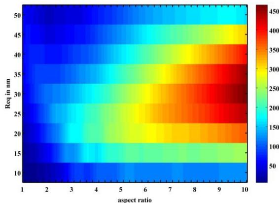
**Figure 1-** BEM-calculated temperature of gold ellipsoids in water, illuminated with a power density  $1\text{mW}/\mu\text{m}^2$  at the LSP resonance wavelength of each object. The temperatures (color) are plotted against the aspect ratios from 1 to 10, and the equivalent radius of the particle (i.e. the radius of the sphere having an equivalent volume).
