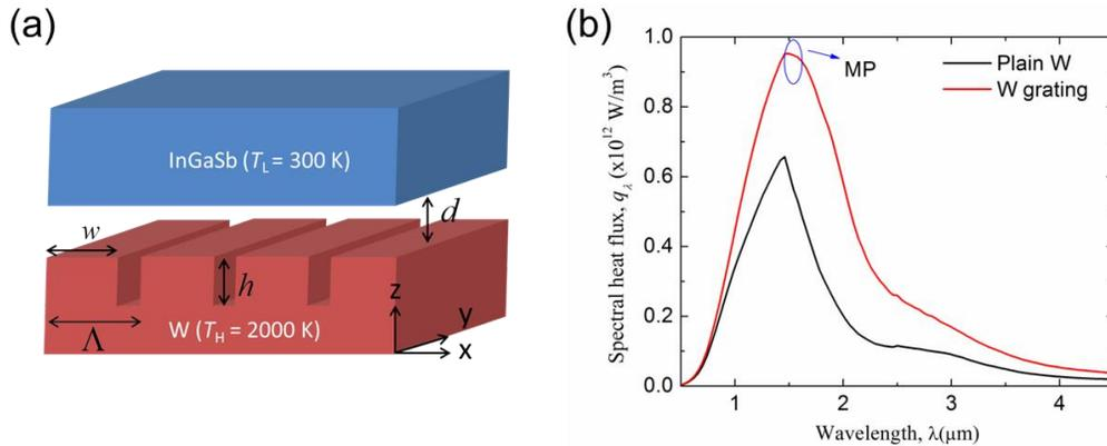
Figure 1. (a) Schematic of the near-field TPV system with an InGaSb cell and a tungsten grating emitter. (b) The spectral heat flux between the TPV cell and plain tungsten (W) or tungsten grating emitter at a gap of 100 nm.
