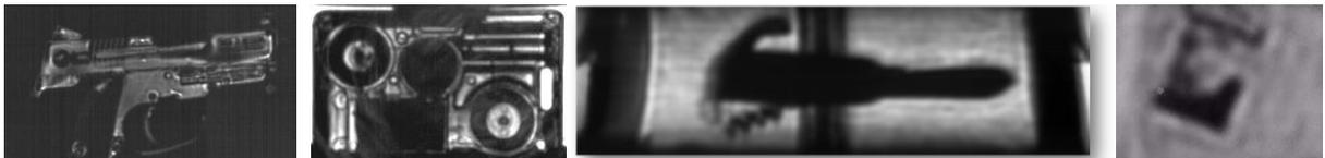
Figure 4. Images taken with the IRXCAM-THz-384: a plastic gun in reflection (left) and a magnetic security card in transmission (center left), both at 2.4 THz; a pocket knife through a leather purse in transmission at 0.69 THz (center right) and a plastic bag filled with water inside a cardboard mailer at 0.29 THz in transmission (right)
